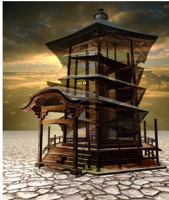
Figure 11: Rendered model: fully rendered internal helical structure with transparent external view superimposed.
