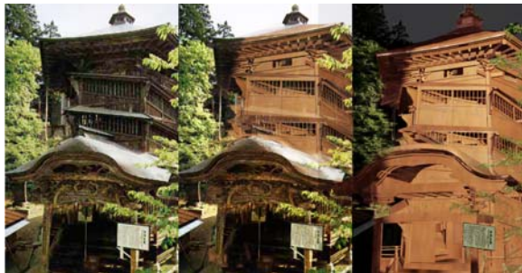
Figure 8: Entrance canopy: (L) photograph; (M) photograph and rendered model merged; (R) rendered model.
