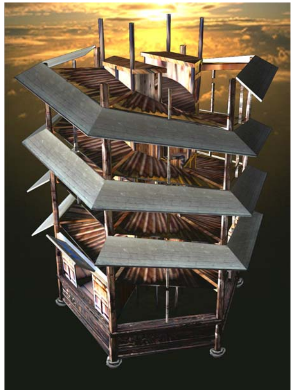
Figure 5: Exterior tower's double-helical exterior overhangs and interior walkway with exterior walls removed; textured model by B. Britton [Bri01].
